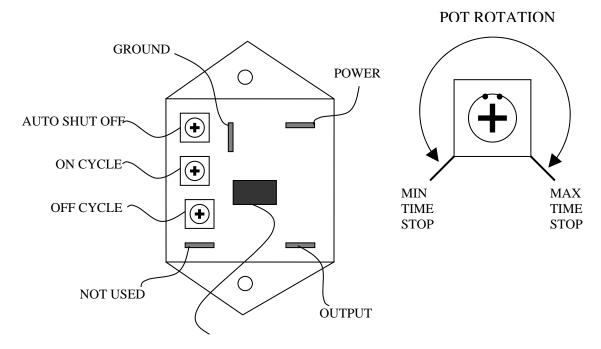
LEAVE THIS CONNECTOR COVER ON OR DAMAGE TO THE TIMER IS POSSIBLE
